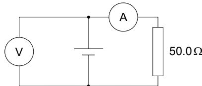
(a) The current in the ammeter is  $59.0\text{ mA}$ .
