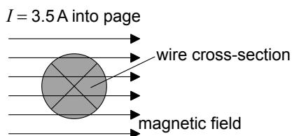
The wire which carries a current of 3.5A into the page, is placed in a region of uniform magnetic field of flux density 0.25 T. The field is directed at right angles to the wire.
