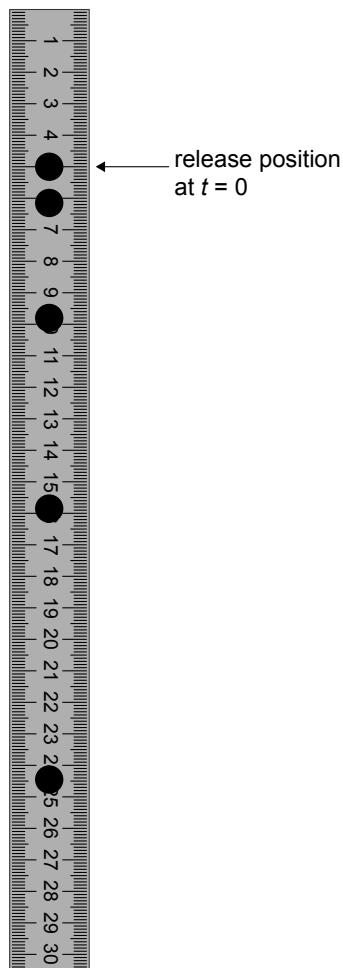
The distance  $s$  fallen by the ball is related to the acceleration  $g$  of the ball and  $t$  by  $s = \frac{1}{2}gt^2$
