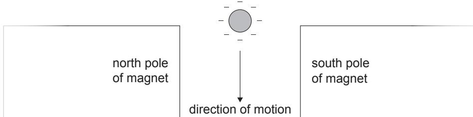
What is the direction of the magnetic force acting on the sphere?
