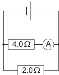
What is the current passing through the  $2.0\Omega$  resistor?
