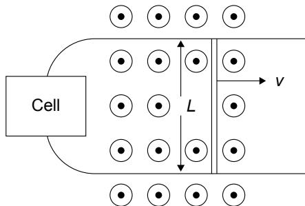
What is the direction of the current through the circuit and the initial force on the metal rod?
