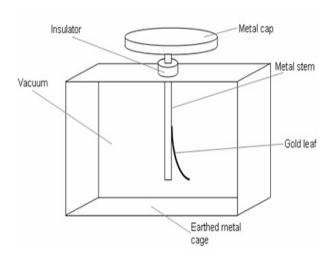
1) Explain what happen to the gold if an rod with a positive charge is brought near the electroscope, without touching the metal cap.
